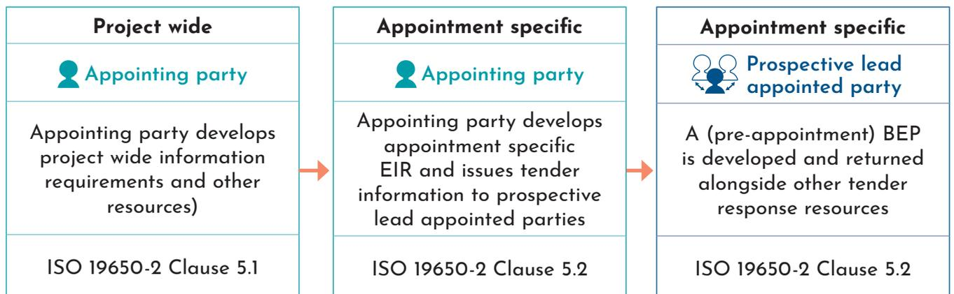
Figure 22: Simplified process leading up to the (pre-appointment) BIM Execution Plan
